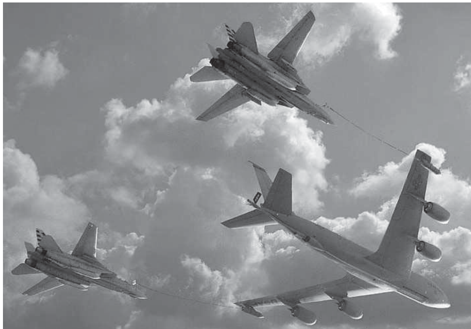
A KC-135 Stratotanker from McConnell AFB, Kan., refuels two U.S. Navy F-14 Tomcats with the Multipoint Refueling System, a configuration that permits the refueling of aircraft not equipped to receive a '135's boom.
