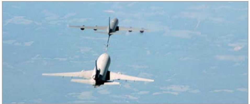
A KC-10 Extender takes on fuel from a KC-135 Stratotanker crewed by the 18th Air Refueling Squadron. (Air Force Photo/Staff Sgt. K.L. Kimbrell )
