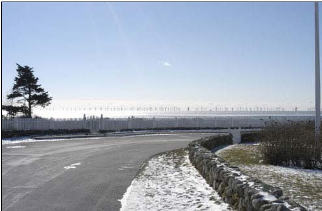
Computer simulation: Cape Wind WTG park as viewed from Hyannis Port, slightly west of Kennedy Compound (viewpoint distance from WTG=5.97 miles; camera elevation=22.44 feet; turbine paint color=off white). Environmental Design and Research ( http://www.saveoursound.org/site/PageServer?pagename=CapeWind_Threats_View ).
