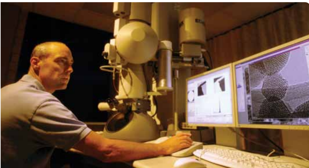
Ames Lab scientist Matt Kramer operates the Lab's transmission electron microscope. Various equipment options allow scientists to probe different aspects of a material. In scanning mode, or scanning transmission electron microscopy (STEM), the electron beam is scanned back and forth across the sample.
