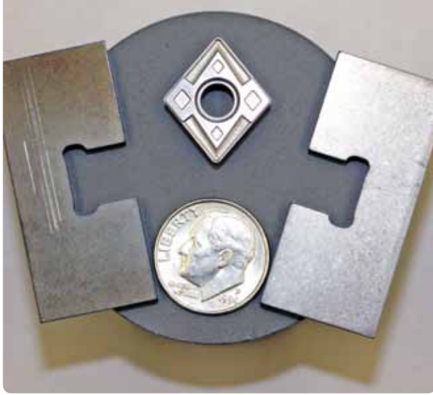
Industrial cutting tools sit atop a disk of the boron-aluminum-magnesium alloy. Even a microns-thin coating of BAM greatly increases the useful life of cutting tools.
