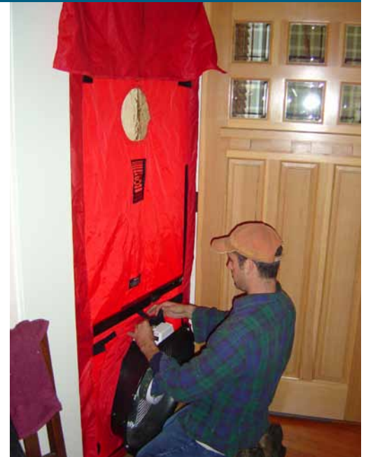
After energy-efficiency improvements are done, the house is tested out with a blower door, duct leakage, and other tests to make sure the home’s energy performance has been improved and that safety standards are met.
