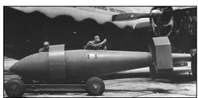
Azimuth Only (TARZON) bomb program combined the 12,000 pound British *Tall Boy* bomb with radio controls in the bomber. The bombardier radioed flight corrections to the bomb based on visual sightings or on television sightings from a camera in the nose of the weapon.
