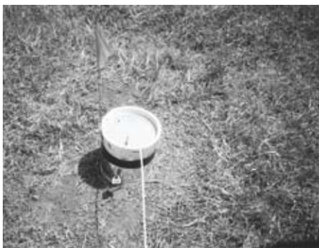
Figure 6. Photograph of equipment used to collect nitrous oxide gas.
