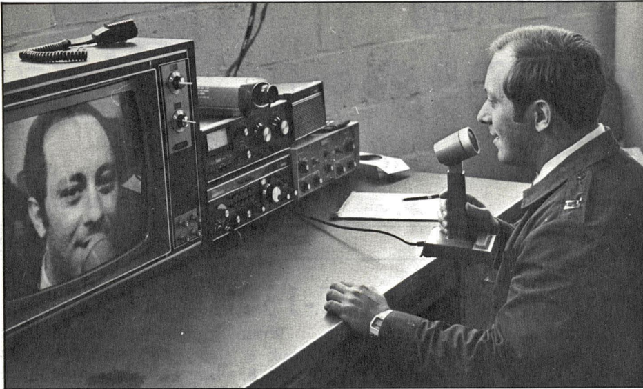
Capt. Jack Sanocki, 905th CF maintenance officer, demonstrates TV reception via high frequency radio to members of his flight.
