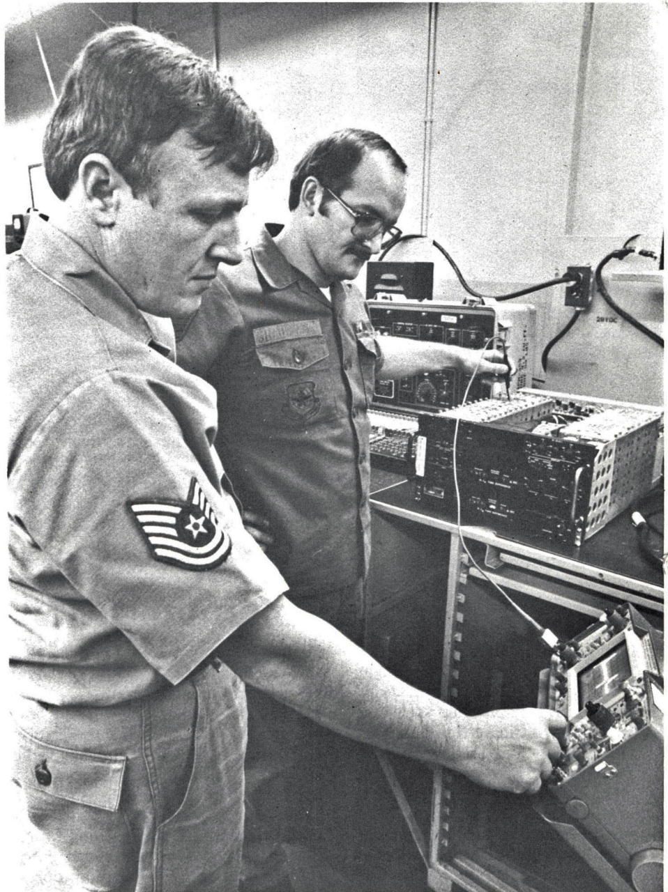
TSgts. Victor Gobbi and William Grabowski, 439th Avionics Maintenance, use an oscilloscope to trace a circuit of an APN-157 LORAN receiver.
