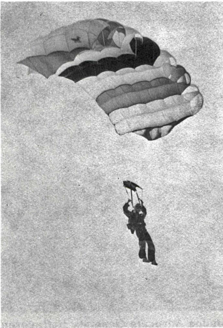
In order to land properly, Sergeant Olszewski 'flares' her canopy which breaks her forward speed.
