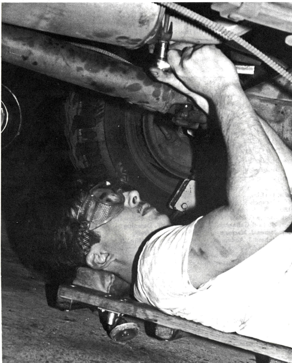
Amn. Dino Panetta replaces the tail pipe of one of the 439th's fire trucks.
