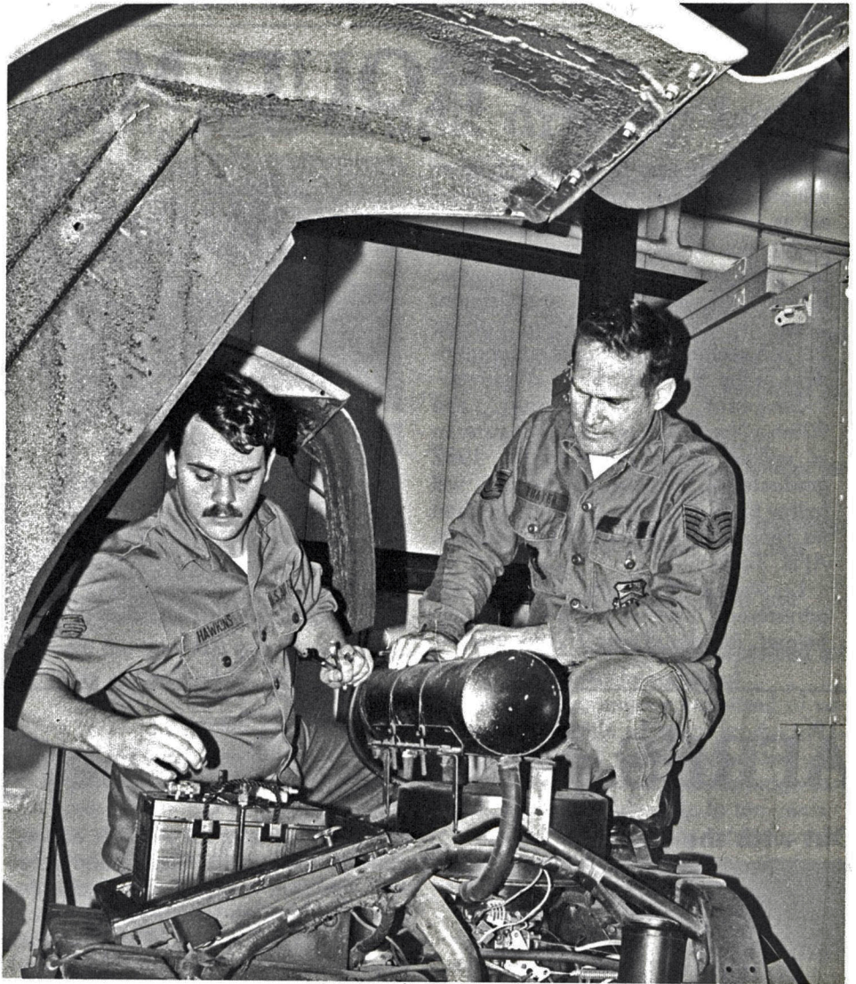
A1C Scott Rindfleisch, left, and Amn. Eunice Langlois repair the alternator of an Air Force truck.
