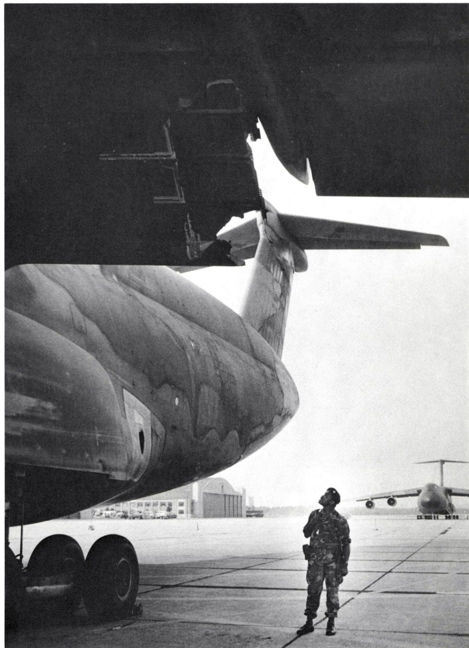
FLAP SHREDS — Sgt. Herman W. Jones examines the shredded wing flap of a C-5A at Westover. When the flap shredded in flight, the metal dropped on a warehouse area in Springfield.
