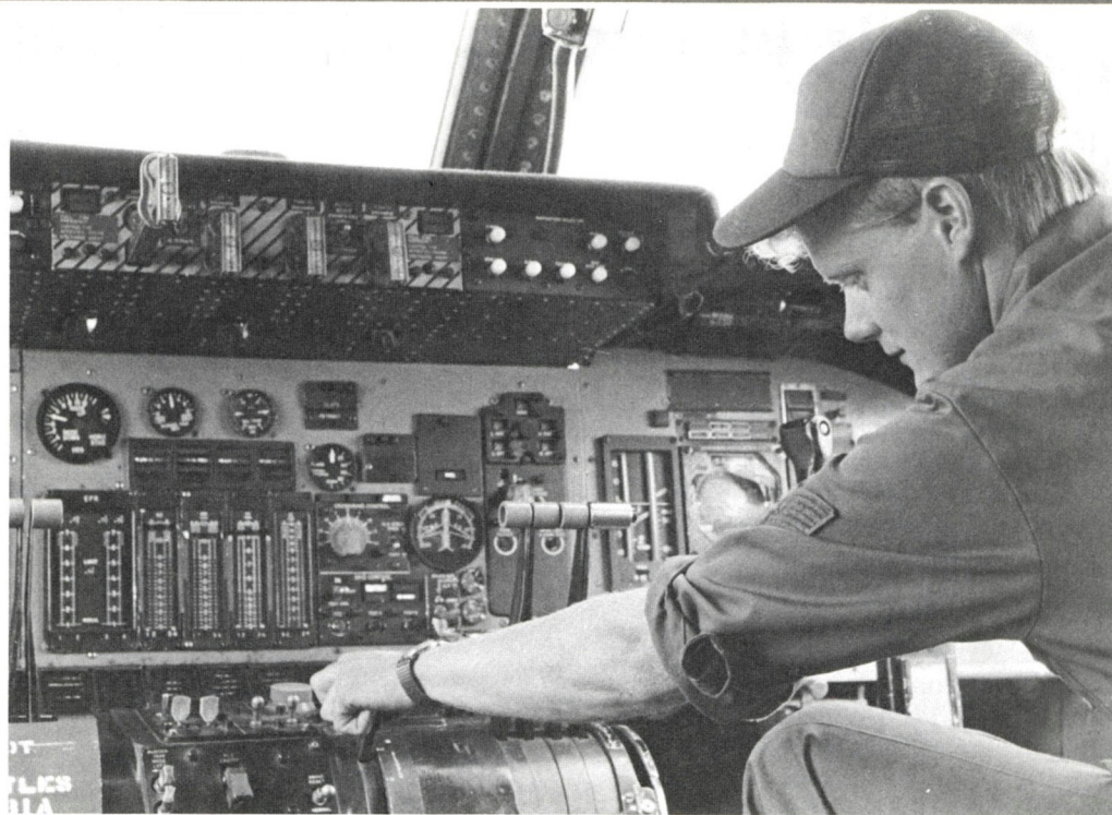
POST FLIGHT INSPECTION — SSgt. Scott Malone, flight line assistant crew chief, lowers the flaps and slats on the C-5 for basic post flight inspection. (USAF photo by TSgt. Sandi Michon)
