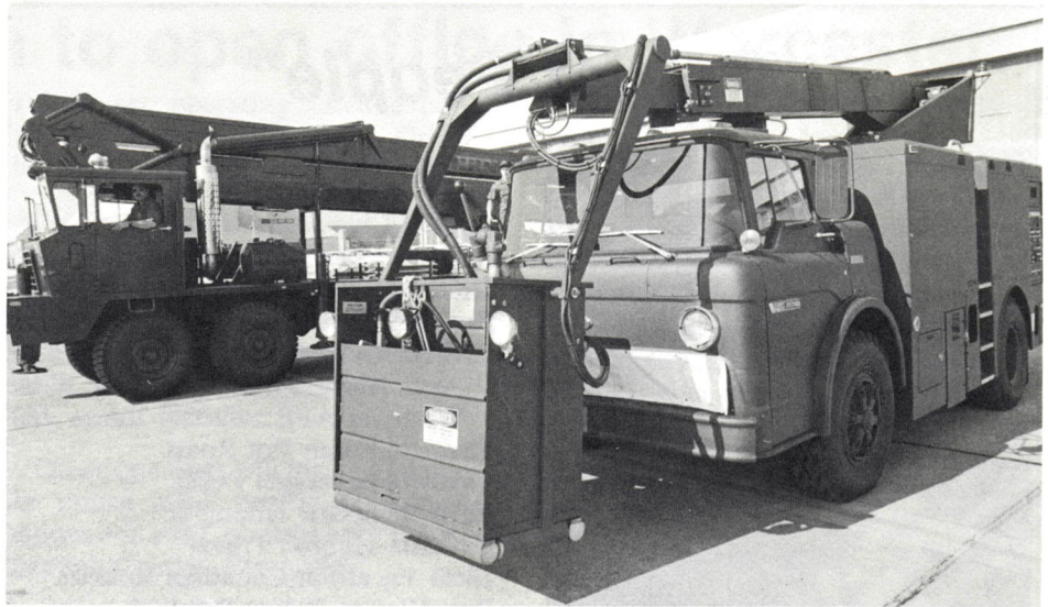
READY FOR SERVICE — SSgt. Paul Gagnon pulls Westover's new Calivar extended bucket reach vehicle (left) next to the Landoll de-icer. When used together, the Calivar's great reach enables de-icing of even the C-5's 65-foot tall tail. The Calivar is the newest addition to the base's inventory of service equipment for larger aircraft.
