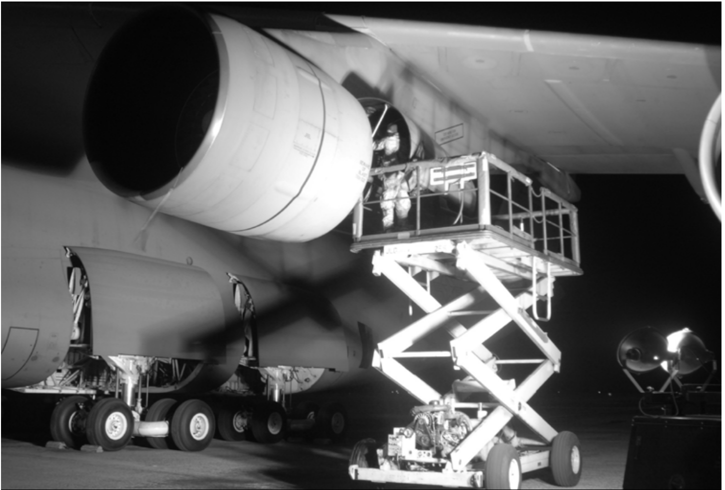
MOBILIZATION >> Senior Airman Zach Allard works late into the night, conducting an oil change on one of the C-5's four massive General Electric TF-39 engines. The Patriot Wing moved to 24-hour operations in support of Operation Enduring Freedom, in April. Westover's C-5B aircraft are providing 35 percent of the Air Force's C-5 missions. (photo by Tech. Sgt. Timm Huffman)
