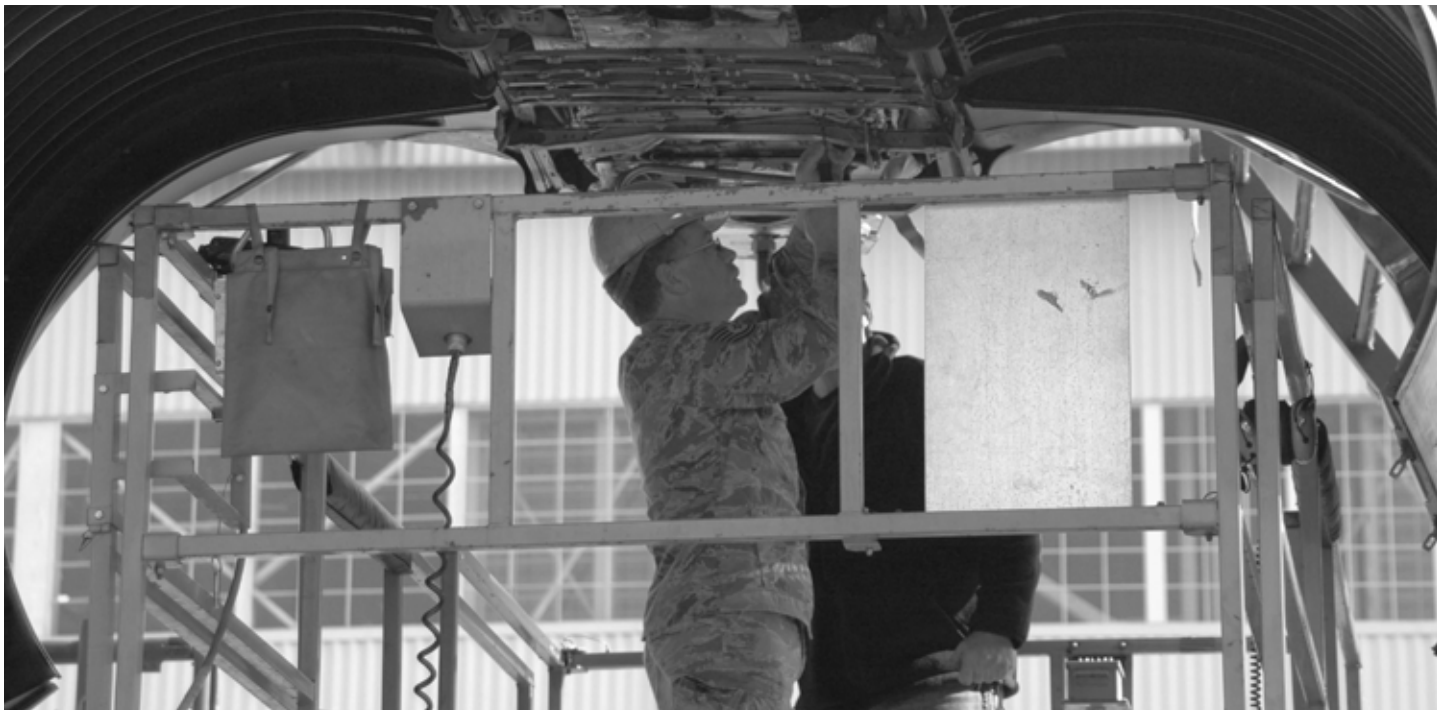
ENGINE CHANGE >> Tech. Sgt. Frank Manegio, 439th Maintenance Squadron Air Reserve Technician, works on a C-5 during an engine change at the isochronal (ISO) area. (photo by Senior Airman Andre Bowser)
