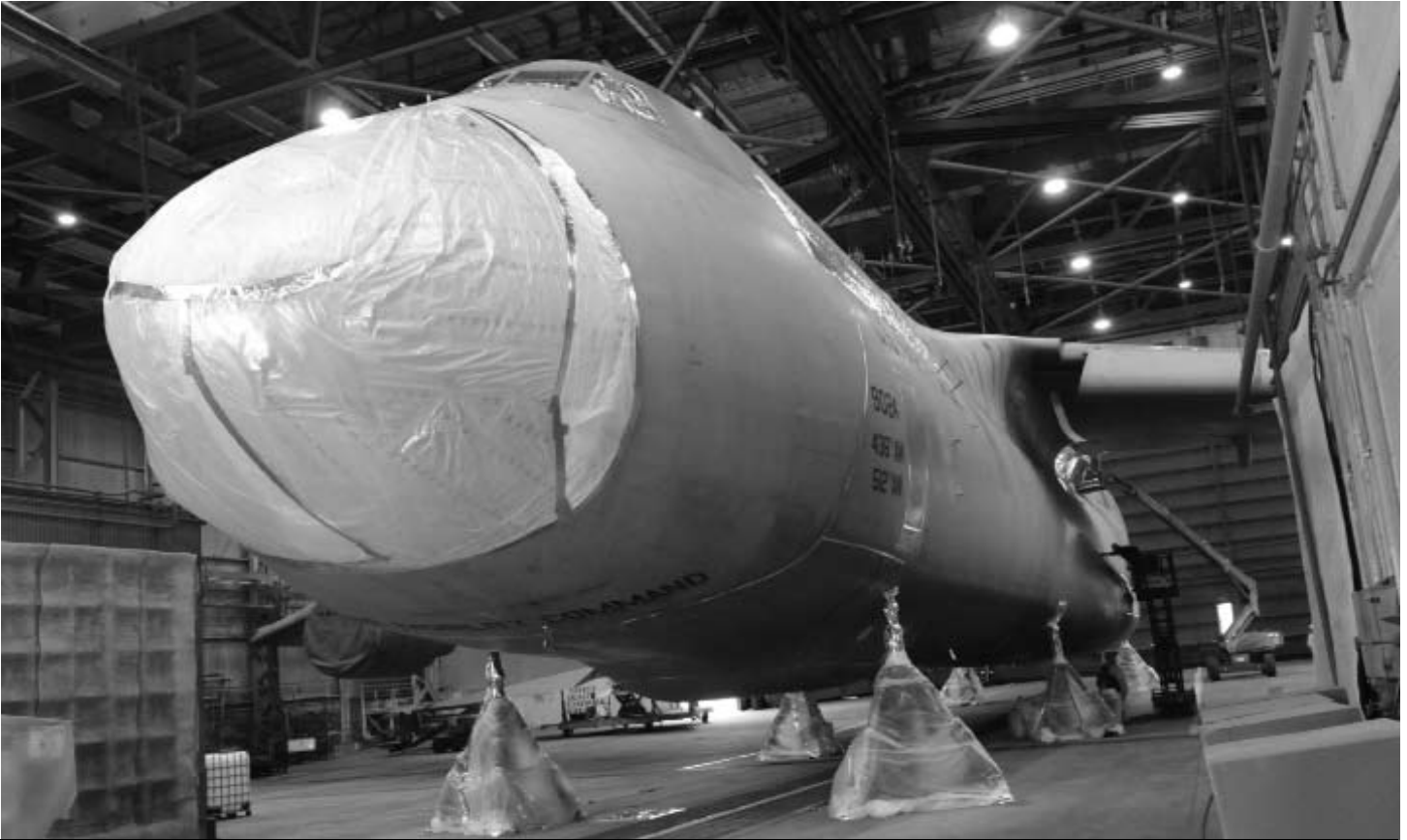
NOSE MASK >> A C-5 sits in a depaint hangar at the Lockheed Martin facility in Marietta, Ga., where workers have masked the seams, composite areas and antennas in order to spray on stripper to remove the paint from the aircraft. C-5s are undergoing Avionics Modernization Program and Reliability Enhancement and Re-engining Program upgrades, modifying them to C-5M Super Galaxys. (photo by Sue Sapp)
