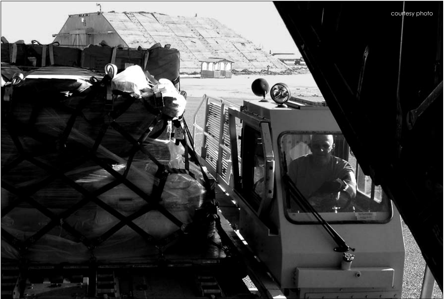
UPLIFTING >> Tech. Sgt. Thomas G. Wilk, 42 nd APS, uses a Next Generation Small Loader to stack pallets on a C-130 at an airbase in Southwest Asia. The base is a main hub for cargo and passengers in and out of Iraq and Afghanistan.
