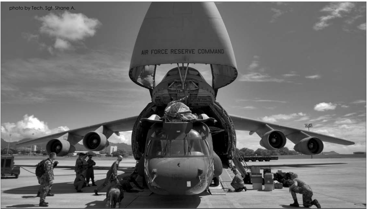
COPTER CARGO >> Air Force Reserve and Army soldiers load two CH-47 Chinook helicopters into a Westover C-5 at Hickam Air Force Base, Hawaii, Oct. 16.
