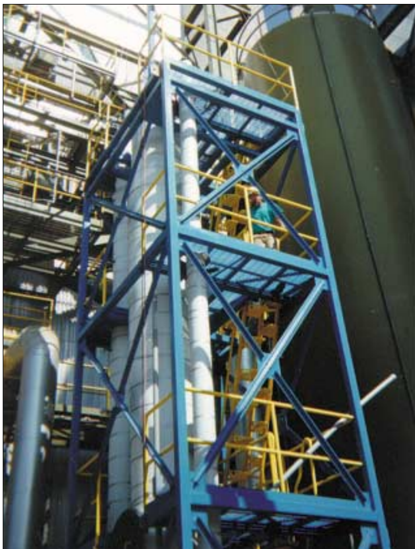
DOE, EPRI, and Public Service Company of Colorado are evaluating carbon injection as a mercury control option on a 600-actual cubic feet per minute test rig located at Public Service of Colorado's 350-MWe Comanche facility
