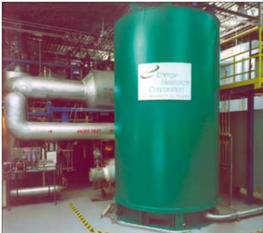
FuelCell Energy's first commercial prototype 250-kW MCFC full-size stack demonstration unit
