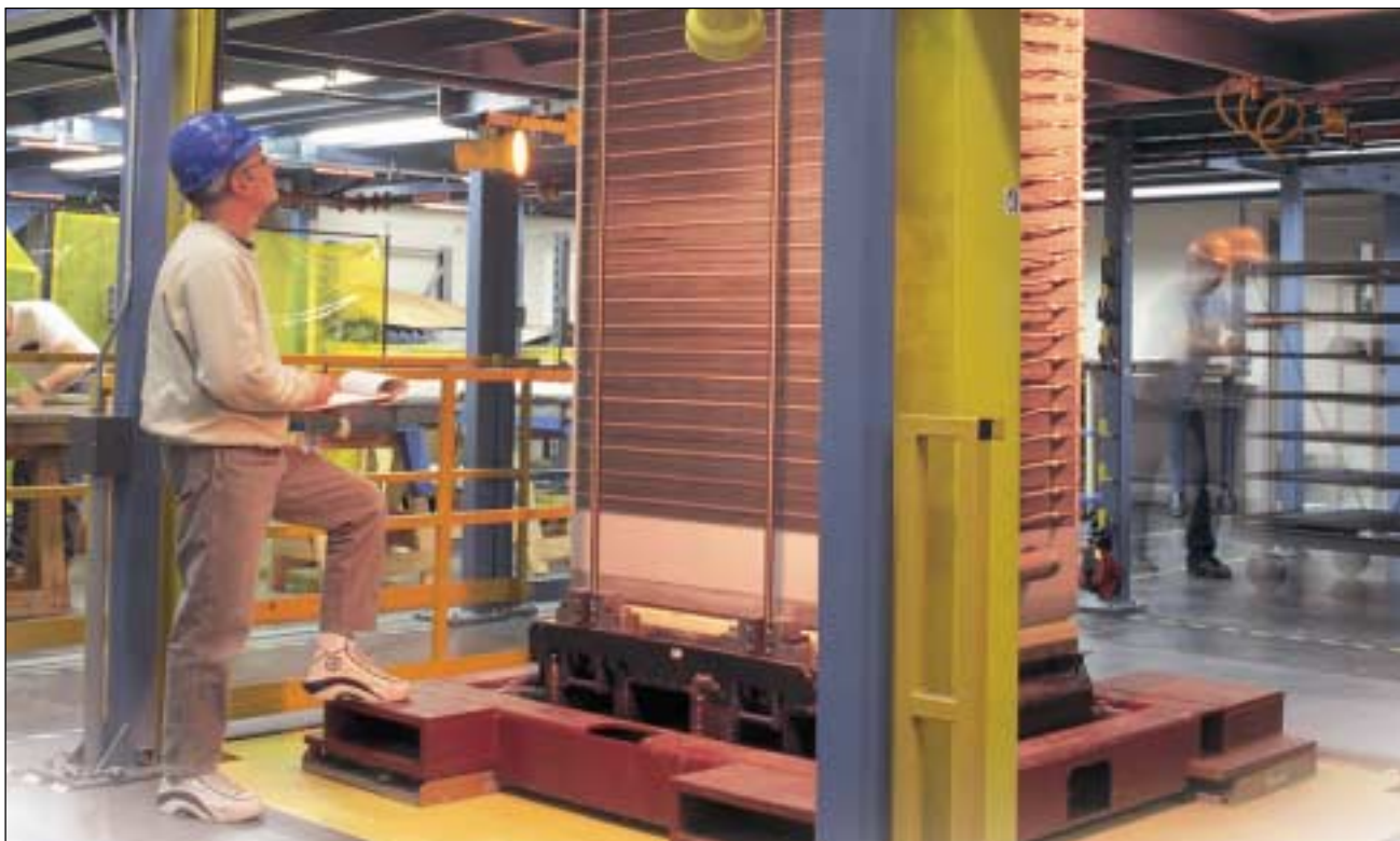
A FuelCell Energy (formerly Energy Research Corp) molten carbonate fuel cell
