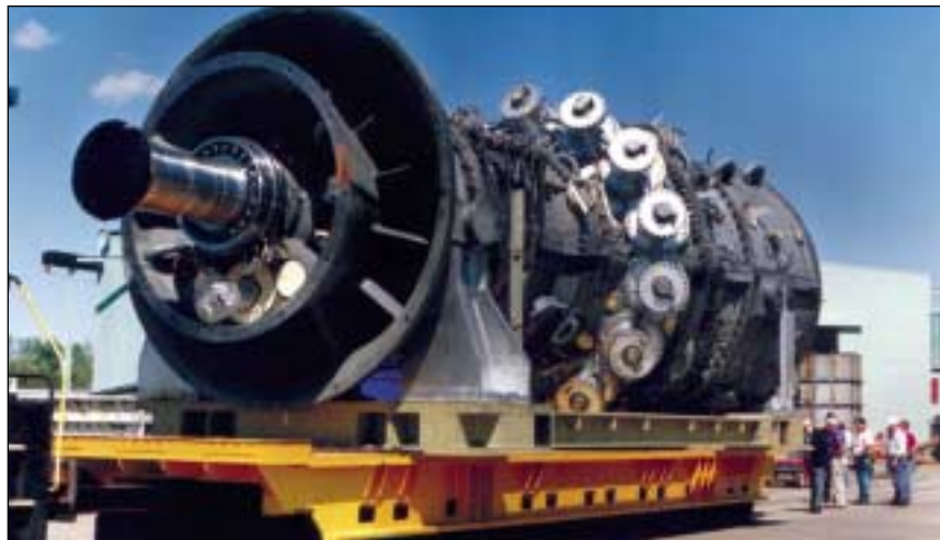
The 400-ton Model MS7001H (H System™) turbine is the size of a locomotive
