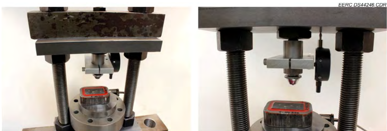
Figure 4. Brinell hardness test equipment and prepared sample specimen.
