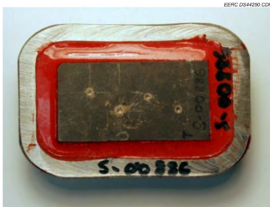
Figure A-2. Rock sample (posttesting) epoxied in a steel ring to assist in sample competency without giving it any drastic increase in strength.
