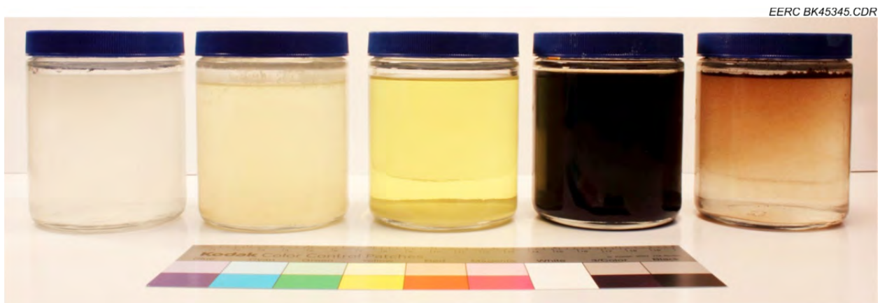
Figure 3. Fluids (from left to right): slickwater, cross-linked gel, gelled diesel, Bakken crude, and Bakken Formation water (brine).
