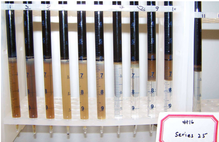
Figure 3.1: Low solubilization of oil and water and gels from tube 8 to 11 observed for Series A25, a ratio 3:1 of Petrostep S1 to Petrostep S2 at 1 wt% total surfactant concentration and 1.5 wt% SBA with Trembley crude oil @ 46.1 °C after equilibrating for 63 days. Salinity varied from 2.0 wt% to 5.0 wt% NaCl at 0.30 wt% increments, left to right.
