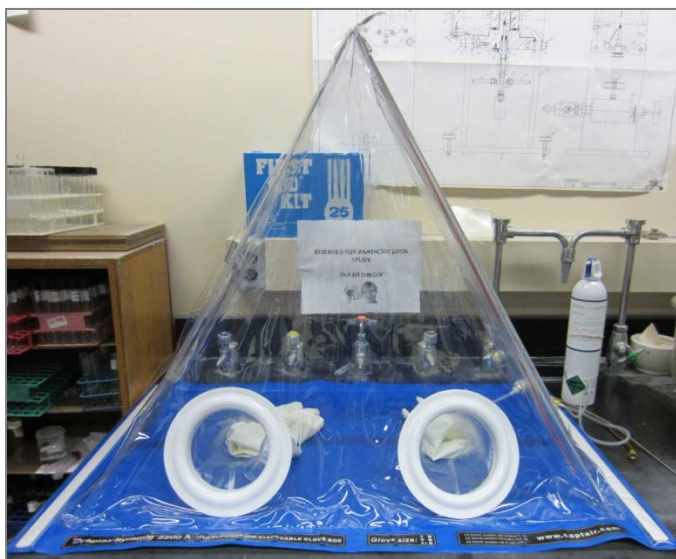
Figure 4-9. Schematic of the nitrogen glove box for the anaerobic experimentation
