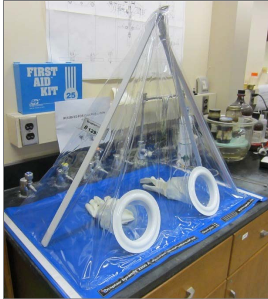
Figure 4-10. Side view of the nitrogen glove box for the anaerobic experimentation
