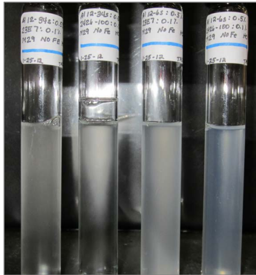
Figure 4-7. Mimic reservoir M brine with no iron with hydrochloric acid
