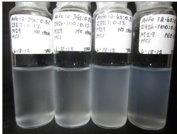
Figure 4-16. Mimic reservoir M brine without iron with hydrochloric acid
