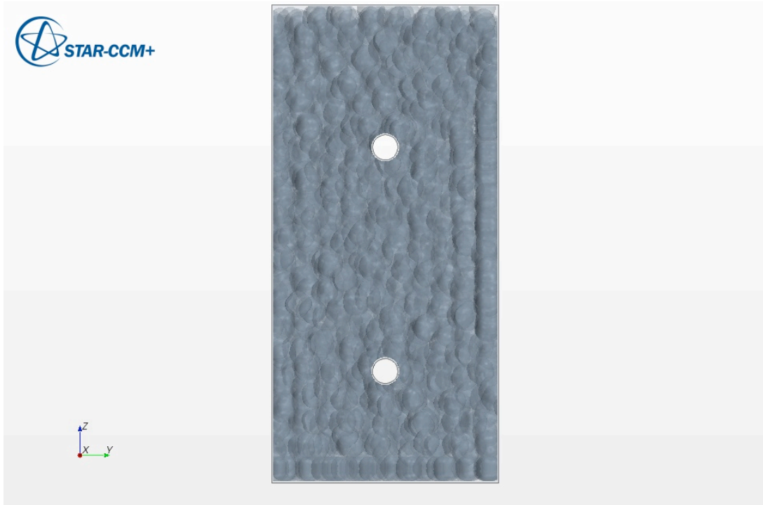
Figure 24. Full size representative computational domain containing about 2,000 oil shale pieces.
