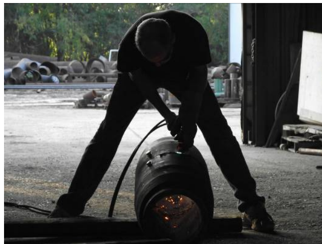
Figure 5.2 – Cutting Samples for Post-Test Examination
