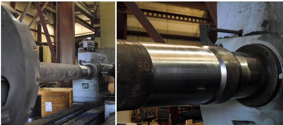
Figure 4.2 – Machining Of Pipe Ends
