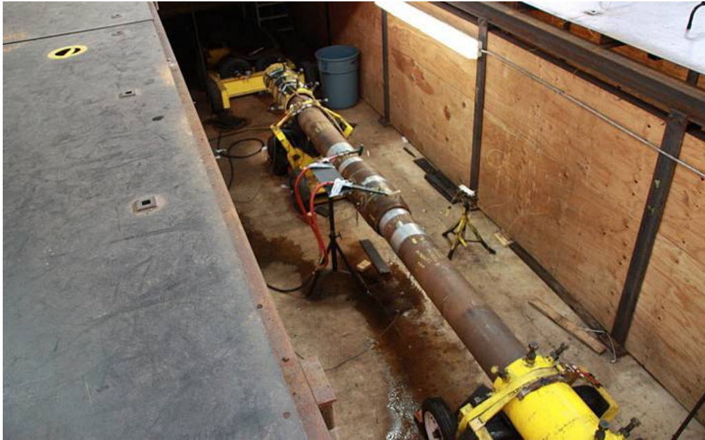
Figure 5.1 – Resonant Bending Fatigue Test Pit, With Sample Installed
