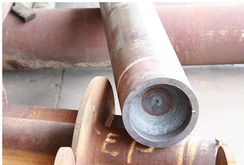
Figure 4.6 – End-Cap Fillet-Weld Into Pipe Bore
