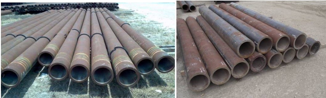
Figure 4.1 – API 5CT SM-C110 Pipe, Before & After Cut to Length
