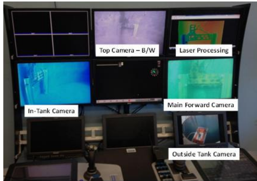
Figure 23. ROV control center. Displays show two ROV mounted cameras, one tank mounted camera, one crane mounted camera, and the laser sensor control screen which is displaying data in the top right screen.
