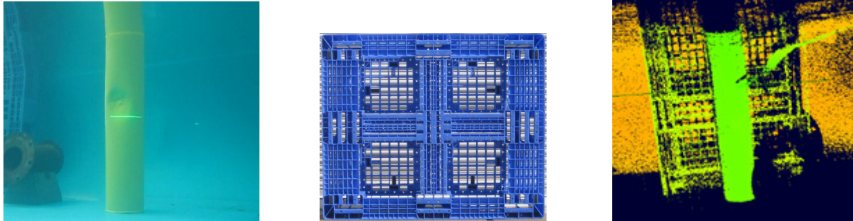
Figure 14. Scan of 8 inch diameter pipe (Left). Blue crate to simulate protective gratings (Middle). Scan with blue crate behind pipe (Right).
