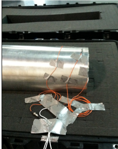
Figure 40. Housing in transit case with three accelerometers attached (one in each axis).
