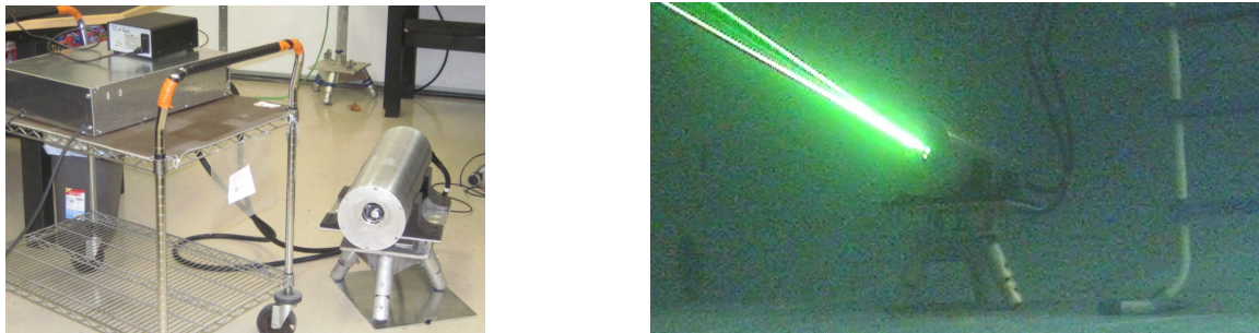
Figure 6. 3D laser sensor on tripod connected to lab power supply on rolling cart (Left) 3D laser sensor and tripod in pool with subsea cables connecting to the lab power supply outside the pool (Right).
