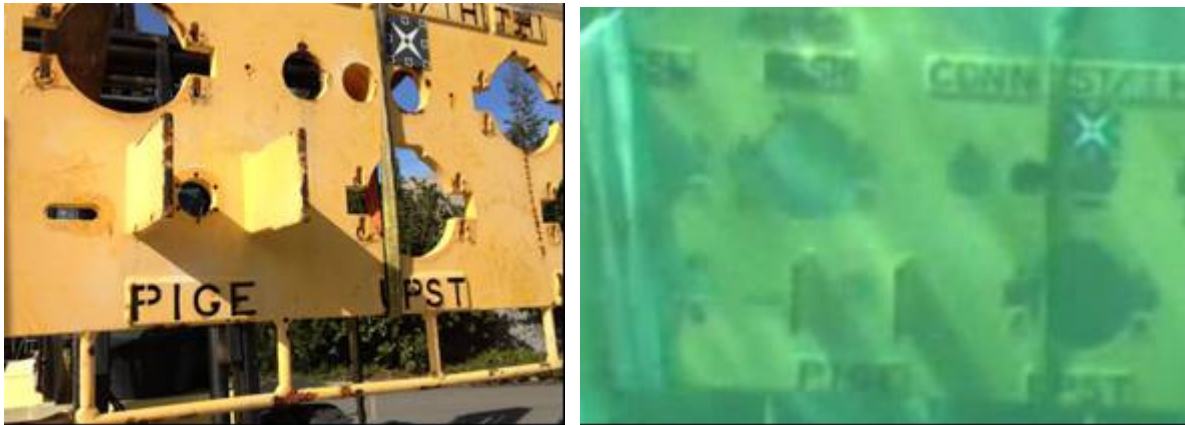
Figure 30. Two fins on the hot stab panel as seen in air (Left) and by the ROV main camera (Right).
