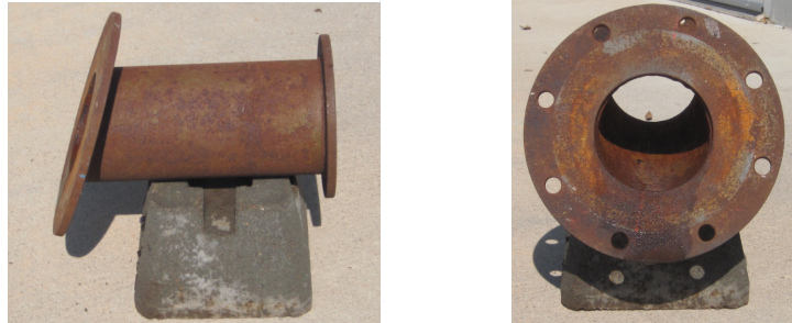
Figure 10. Rusted, angled flange target (Left). The attitude is not identifiable with a straight-on orientation (Right).
