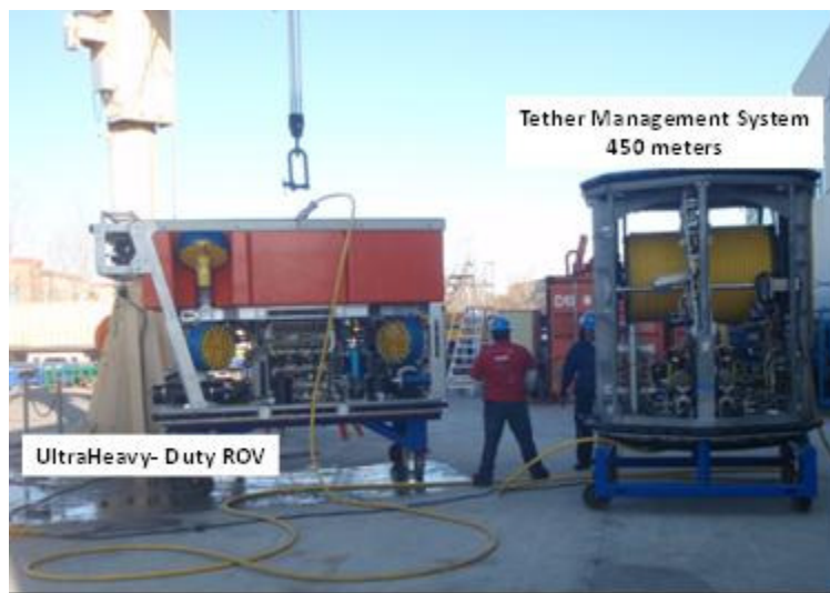
Figure 22. Power and communications are delivered to the ROV through a 450 meter tether.
