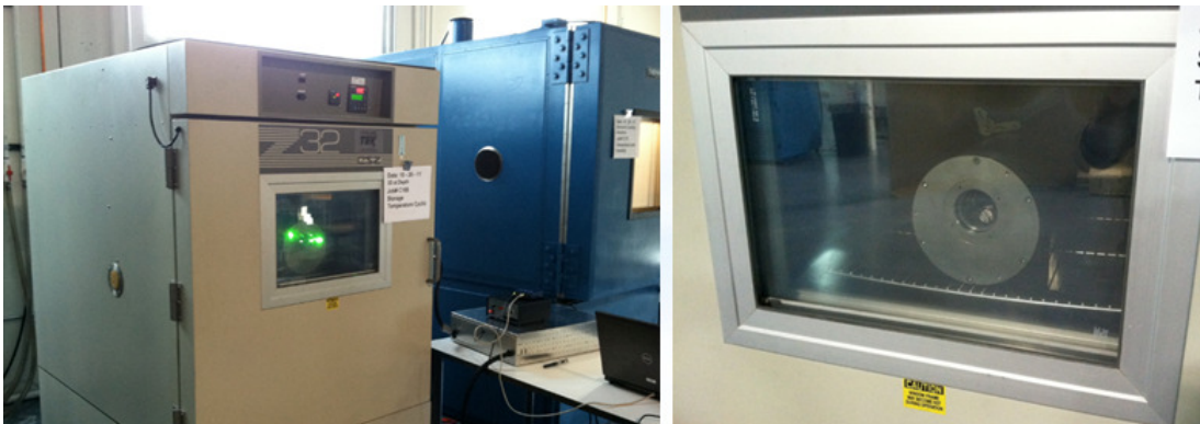
Figure 36. Window in thermal chamber allows functional testing of the sensor during thermal tests.
