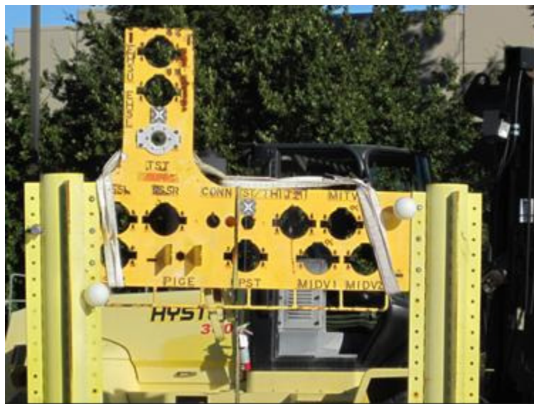
Figure 24. A Hot stab panel was used as the primary target for this test.
