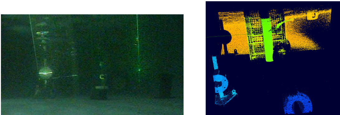
Figure 9. Multiple objects scanned at once. Image from HDTV underwater camera while performing a large area scan (Left). Resulting 3D data where color is mapped to range – blue is short range (Right).
