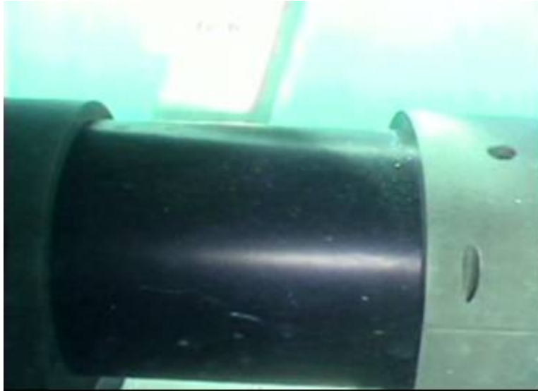
Figure 32. Still-screen capture of the laser sensor from the ROV main camera showing some of the particulates in the water. Every white spot and streak is a particle.
