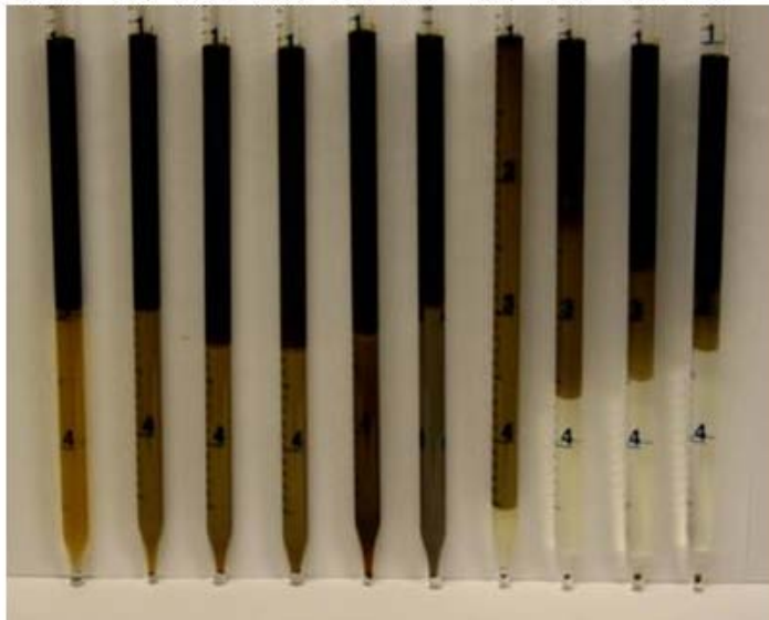
Figure A.9: B-34 Phase Behavior Pipettes after 3 Weeks' Settling.
