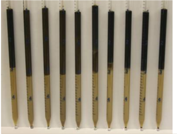
Figure A.7: B-12 Phase Behavior Pipettes after 1 Week Settling
