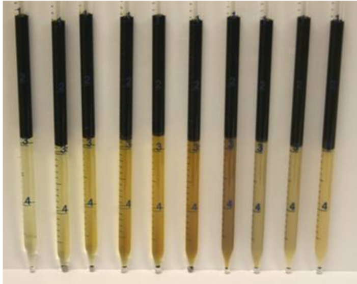
Figure A.8: B-33 Phase Behavior Pipettes after 3 Weeks' Settling.
