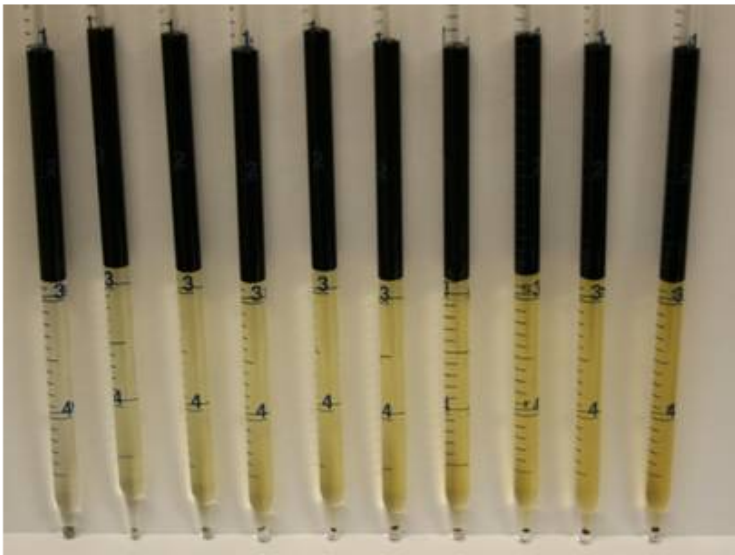
Figure A.6: B-11 Phase Behavior Pipettes after 1 Week Settling.
