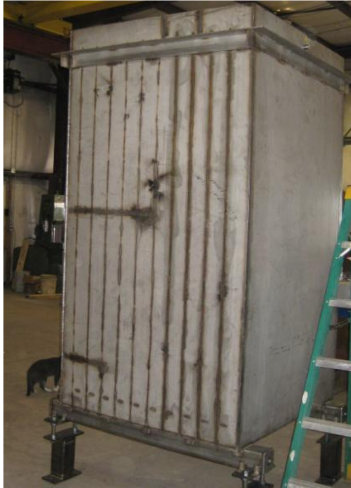
Figure 24: Prototype HDH module in the fabrication shop.
