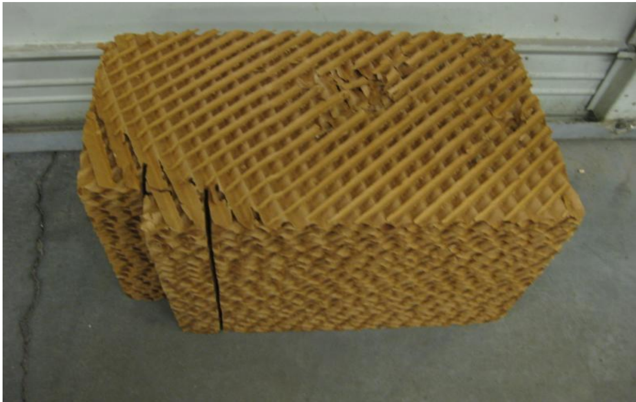
Figure 28: Packing material used inside the humidification chambers.
