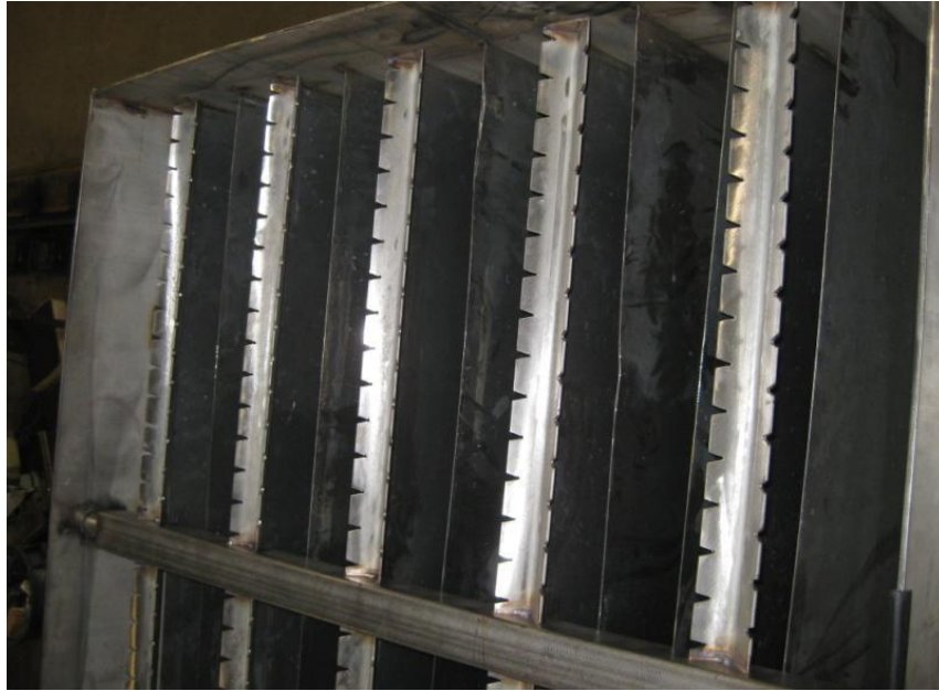
Figure 26: Manifold containing V notched weirs for the water inlet.
