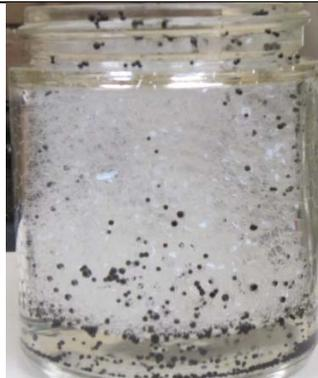
Figure 61. Proppants ULW1 Polymer stay in the foam
