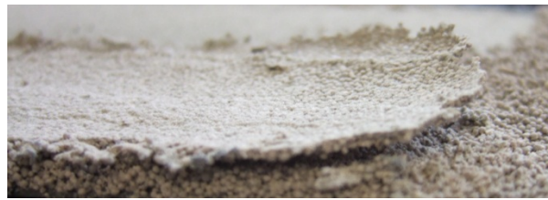
Figure 39—Dehydrated polymer-proppant cake.
