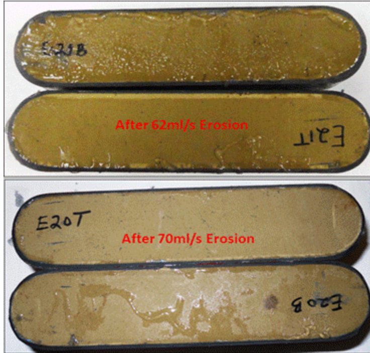
Figure 31—Core surfaces after erosion (cleanup) test.
