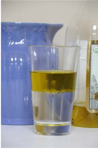
Oil and water form separate phases when mixed.
