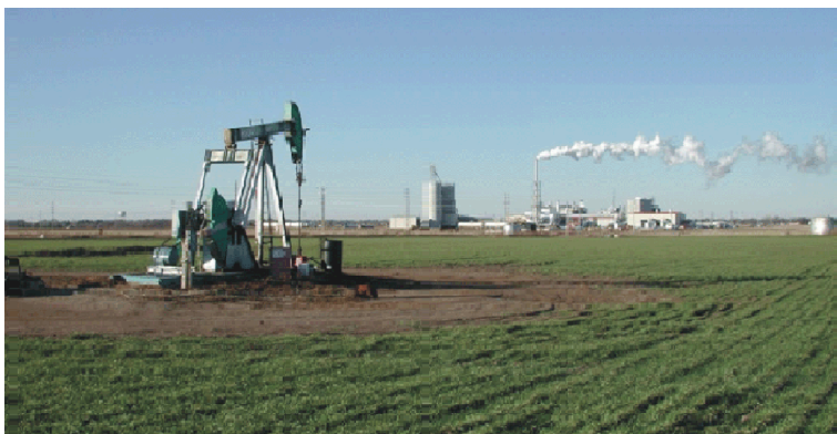
In 2010, NETL demonstrated carbon dioxide flooding EOR in the Hall-Gurney field in Russell Kansas, using carbon dioxide recovered from a nearby ethanol plant.
