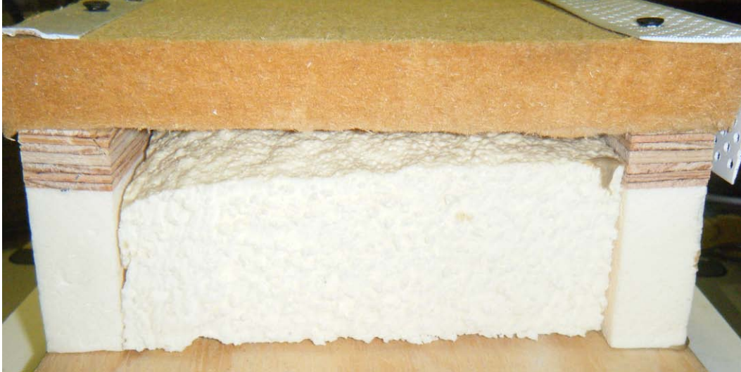
Figure 7. Mock-up of IFT insulation system: two continuous layers of insulation and air gap
