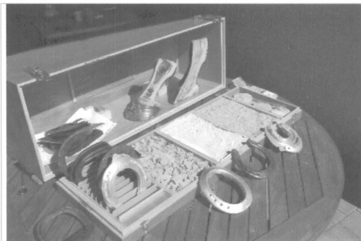
Where the horseshoe meets the footing: I love this display of horseshoes and footing samples used to explain why and how horseshoes function differently on, for instance, soft but firm (synthetic) vs soft and yielding (sand) arenas. Features that enhance a shoe for one surface may be a liability on another. Horse foot shape (especially width) and pastern length and angle also affect how the foot interacts with different surfaces. This is an area deserving much, much more study. (Note Euro rock 'n roll shoe at far right, in front of case.) Photo courtesy of Germany's Loic Entwistle.
