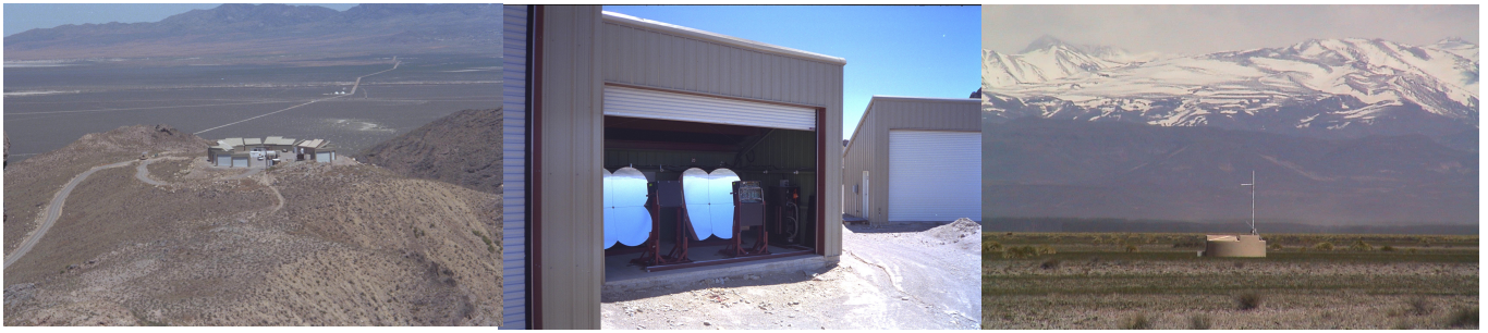
The HiRes observatory lies in the Utah desert, comprising a ring of detectors on two plateaus (left). When the Sun goes down, the doors are lifted to expose the HiRes mirrors (middle). Ultrahigh-energy cosmic rays interacting with material in the atmosphere create a fluorescent disk, which travels downward. This results in the generation of ultraviolet light, which these mirrors reflect onto special detectors. The Auger Observatory, under construction on the high western plains of Argentina, employs similar detectors placed across hundreds of kilometers and also relies on a second kind of detector (right).
