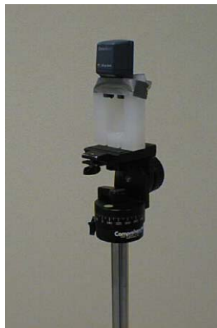
Figure A.3.4. Rotary Mounting for DataSeal
