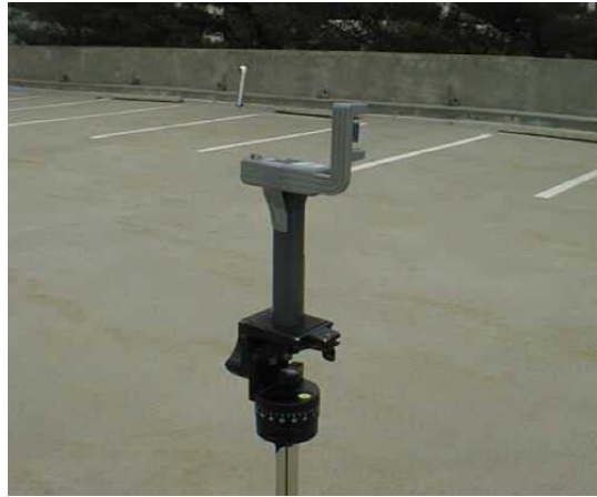
Figure A.4.5. Rotary Mounting for SmartSeal
