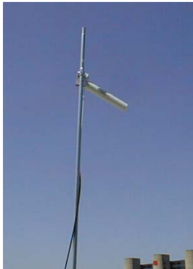
Figure A.5.6. 2.44 GHz Yagi Antenna (with radome) Used to Measure Signal Strengths
