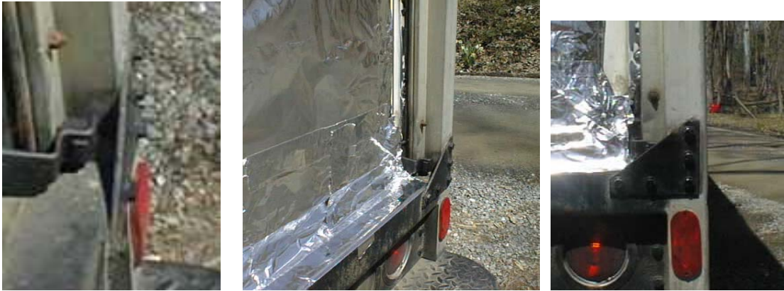
Figure A.5.15. Views of ALL Seal During and After Installation in Door Seam
