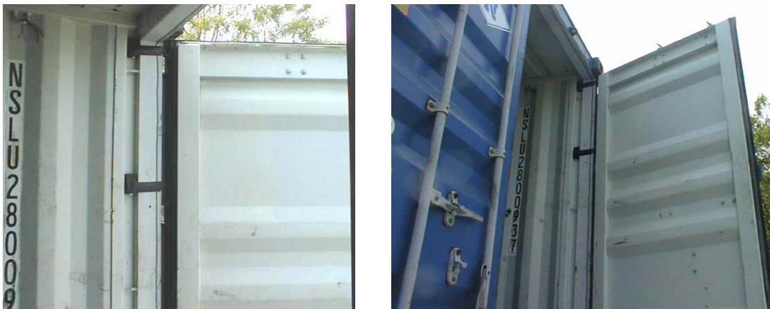
Figure B.30.c. Seals Mounted on Container Frame
