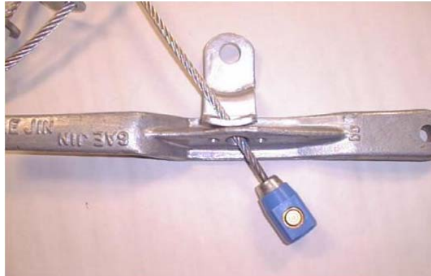
Figure A.6.2. Close-Up of Memory Button Epoxied into a Locking Head
