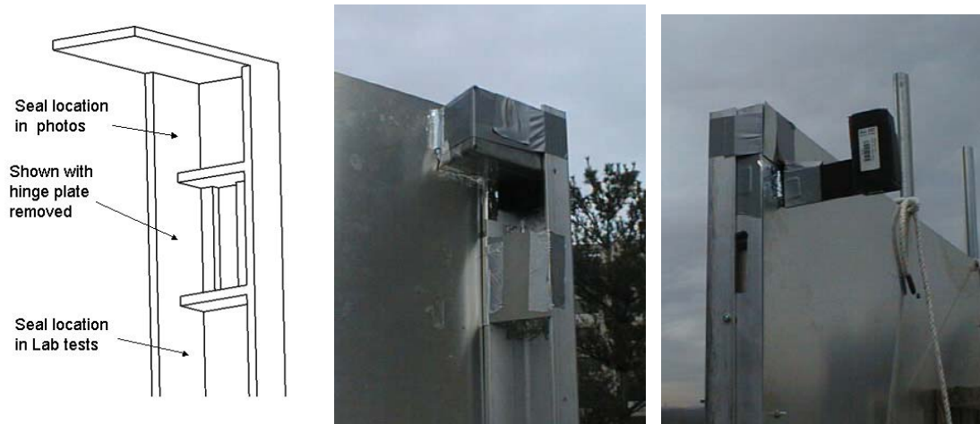
Figure A.5.10. Simulated Hinge Region and Seal Mounting for Lab Tests
