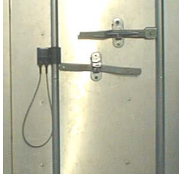
Figure A.3.8. Detail of Simulated Container Door, Handles, and Keeper Bars
