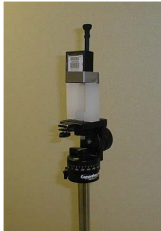
Figure A.2.4. Rotary Mounting for E-seal
