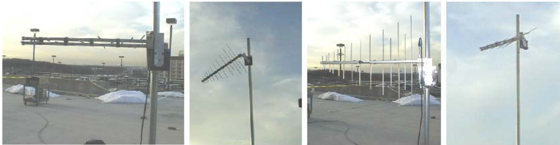
(a) Level, horizontal elements (b) Elevated, “vertical” elements (c) Vertical elements (d) Elevated, “horizontal” elements
