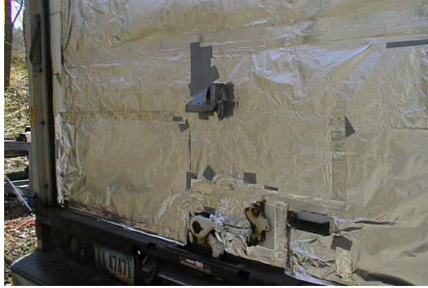
Figure A.4.12. Savi Seal Attached to Coated Roll-Up Door
