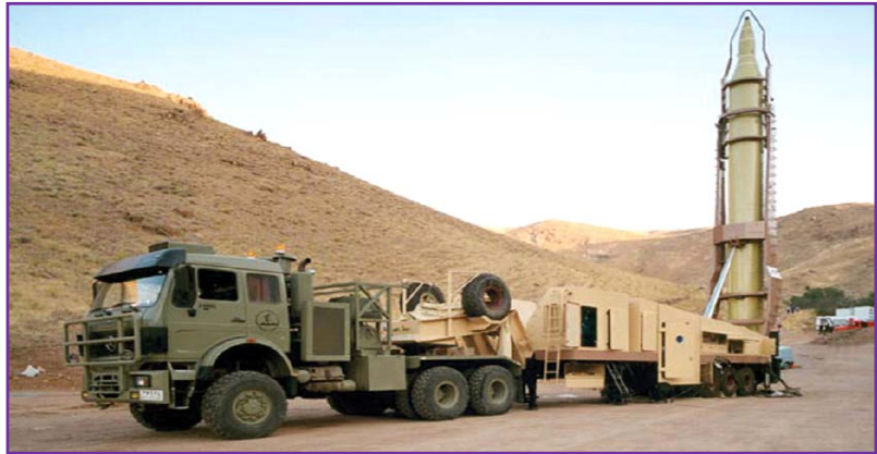
IRANIAN SHAHAB-3 VARIANT MRBM. The Iranian Shahab-3, with a range of 1,300–2,000 km, is a mobile system capable of evasion.
