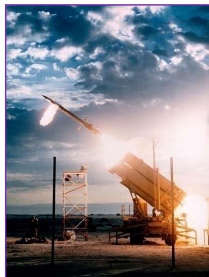
PATRIOT MISSILE LAUNCH. PATRIOT missile defense interceptors are capable of intercepting short- and medium-range missiles at relatively close range in their terminal phase of flight.
