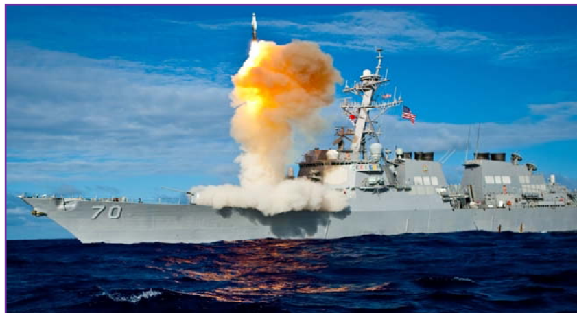
AEGIS BMD SM-3 FLIGHT TEST. The Arleigh Burke-class guided missile destroyer USS Hopper, equipped with the Aegis Weapons System, is shown launching a SM-3 while underway in the Pacific Ocean. The missile successfully intercepted a short-range ballistic missile launched from the Pacific Missile Range Facility in Kauai, Hawaii. This exercise marked the 19th successful intercept of 23 at-sea firings using the Aegis Ballistic Missile Defense System.
