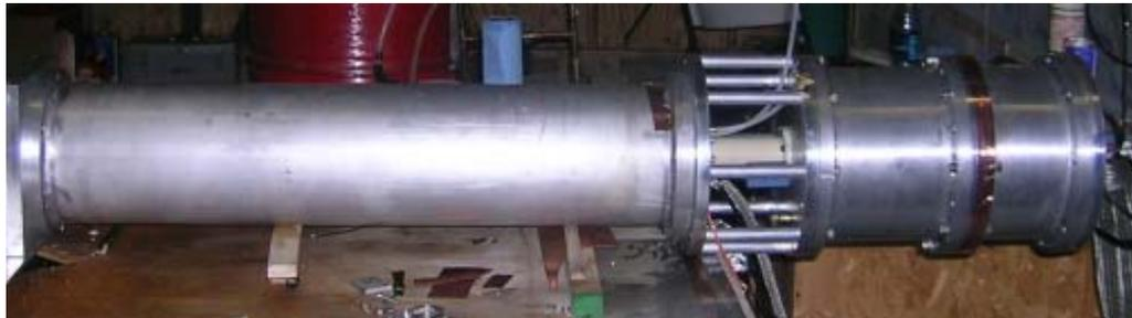
Figure 19. Marx generator and power supply.
