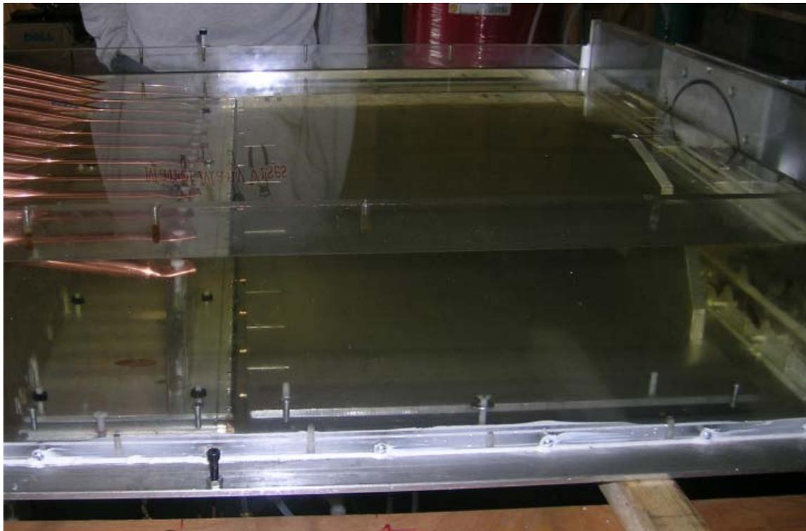
Figure 20. Flat plate Blumlein configuration oscillator subsystem.
