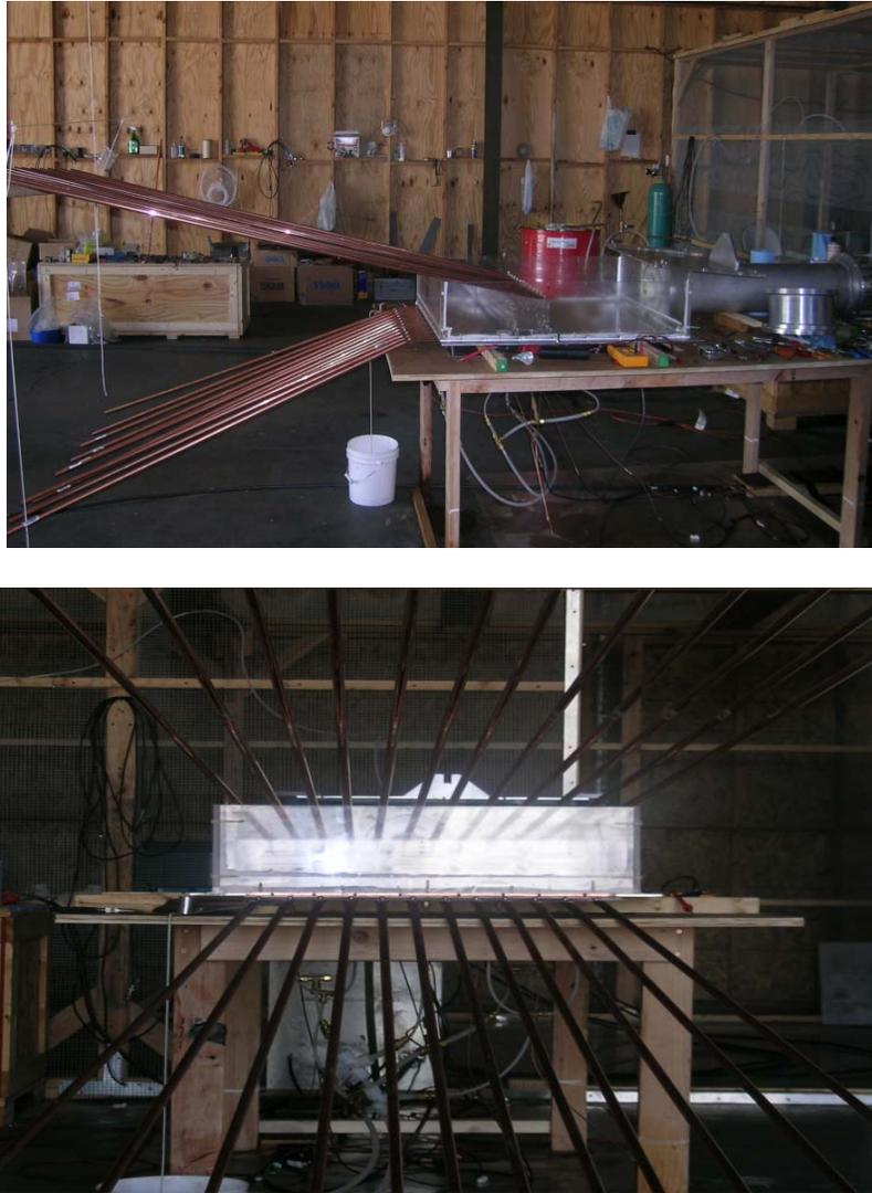
Figure 21. Flare horn antenna subsystem
