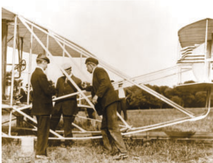
Wilbur and Orville Wright prepare their airplane for flight over Huffman Prairie. Note the American flag on the elevator at the front of the aircraft
