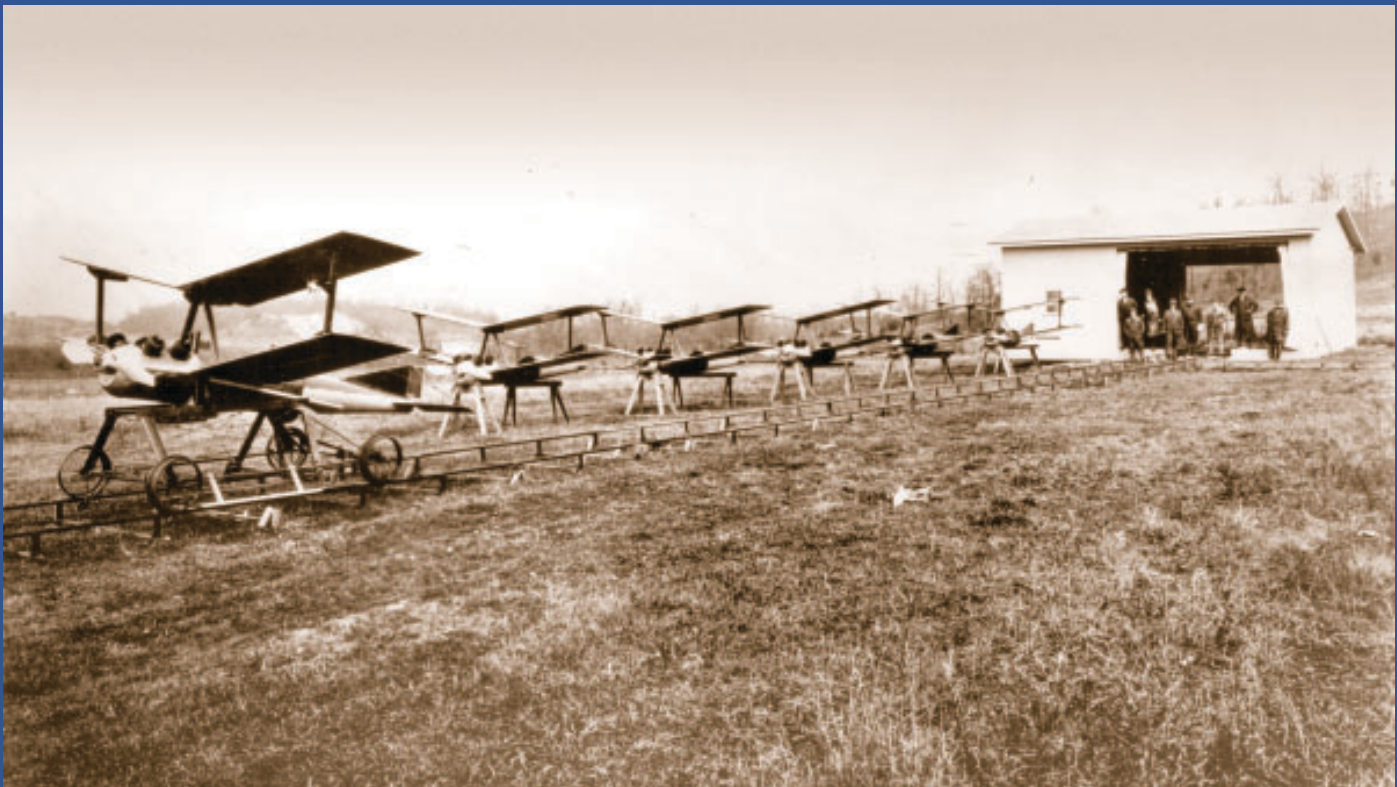
Kettering “Bugs” lined up on their launch rail ( Montgomery County Historical Society )
