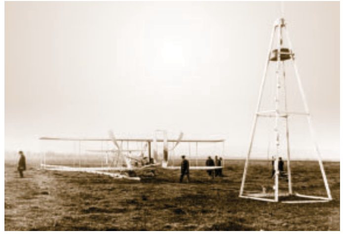
Wright Flyer and the catapult built by the Wright brothers for launches at Huffman Prairie, shown here in Pau, France, 1909. The Wrights traveled extensively to demonstrate their airplane and its flying qualities.
