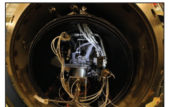
A collaboration between AEDC and graduate students at the University of Tennessee Space Institute (UTSI) resulted in experiments of cryo-contamination in AEDC's small ultra high vacuum (UHV) chamber. This look inside AEDC ultra high vacuum (UHV) chamber shows the equipment used to measure the formation of cryo-deposits, including a mirror and a quartz crystal microbalance (QCM). (Photo by Rick Goodfriend)
