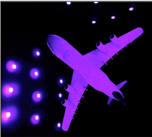
Pictured here is the C-5M Super Galaxy model during a break in testing in Arnold Engineering Development Complex's (AEDC) 16-foot Transonic Wind Tunnel (16T). The model's coloring is a result of the purple Light Emitting Diodes (LED) used to illuminate the Pressure Sensitive Paint (PSP). The over-arching goal of the recent test was to validate the computational fluid dynamics predicted drag reduction effects of winglets on the C-5M, the Air Force's most current version of the aircraft. (Photo by Rick Goodfriend)
