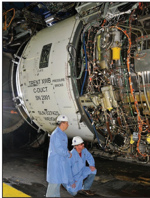
From left, Aerospace Testing Alliance outside machinists Danny Haddon and Garry Sudberry inspect the Rolls-Royce Trent XWB engine between simulated altitude performance and operability test runs in AEDC's C2 test cell. The engine is the largest power plant ever tested at AEDC. (Photo by Rick Goodfriend)
