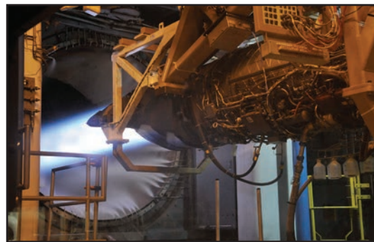
AEDC completed a Continuous Improvement Program (CIP) Life Extension Accelerated Mission Test (AMT) on an F119 engine for the F-22 Raptor in the Sea Level 2 (SL-2) facility. The engine is pictured undergoing AMT testing in SL-2 with the augmentor activated. (Photo by Rick Goodfriend)
