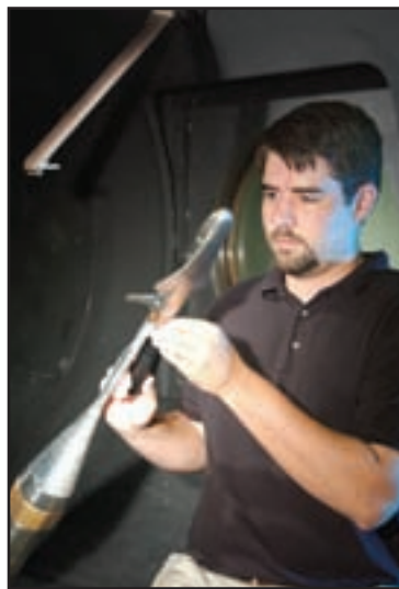
Project engineer Joe Norris puts the finishing touches on the X-37 model prior to testing at Mach 14 in Tunnel 9.
