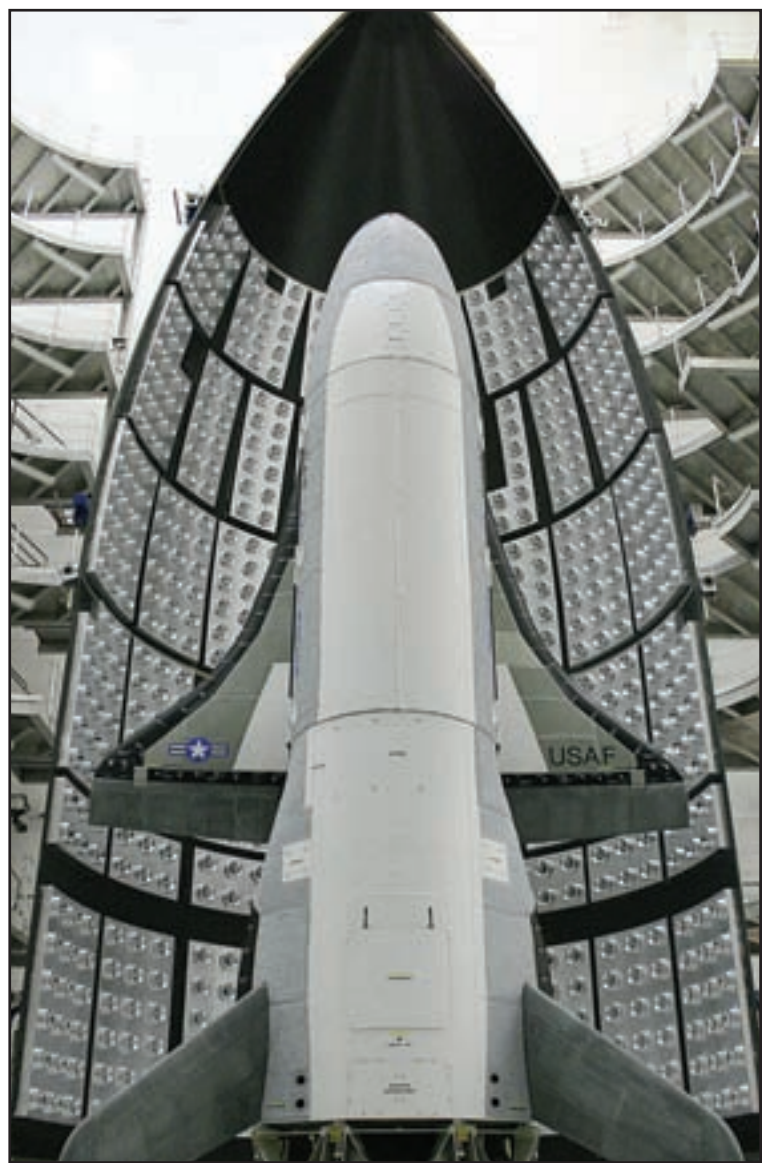
The X-37B Orbital Test Vehicle waits in the encapsulation cell of the Evolved Expendable Launch Vehicle April 5, at the Astrotech facility in Titusville, Fla. Half of the Atlas V five-meter fairing is visible in the background. (Courtesy photo)
