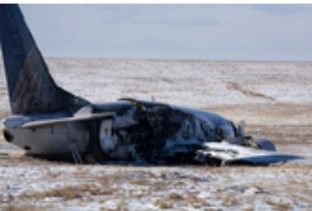
This Boeing 737 airplane was destroyed during a runway excursion when it ran off the runway while attempting takeoff.
