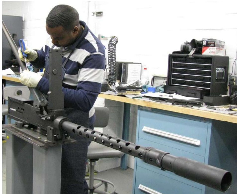
At Gun Point David Forrest of AMCOM's Maintenance Operations Procedures and Prototype facility reassembles a M3P .50 caliber machine gun that was once used on an Avenger air defense system, but will soon be on an OH-58
