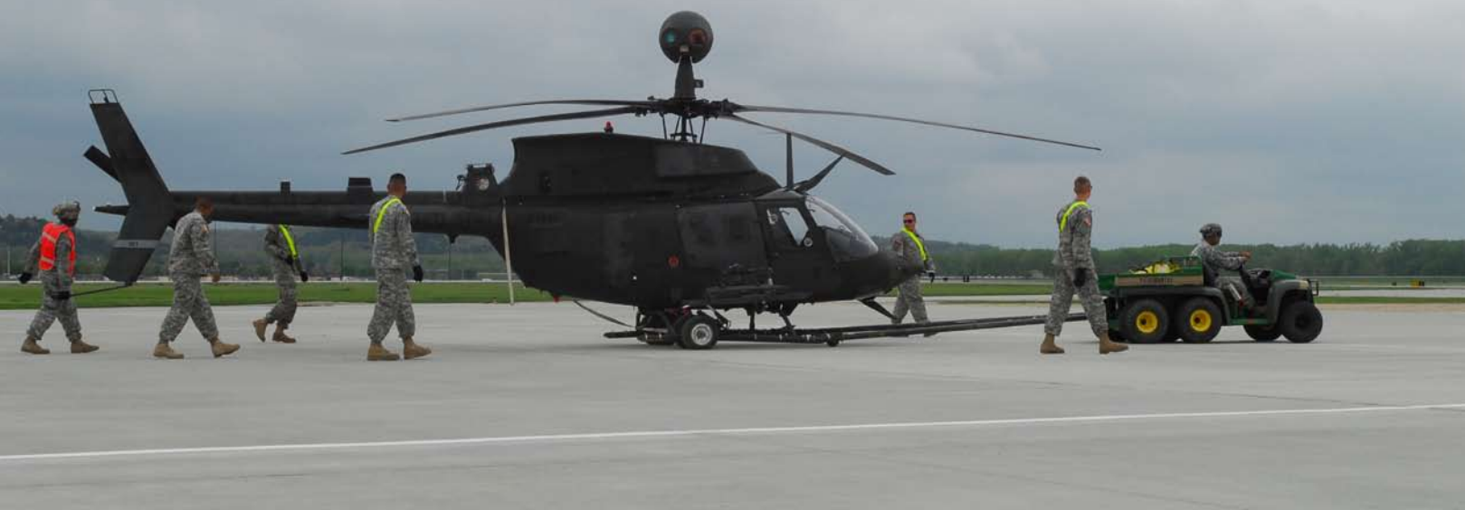
OH Entourage Fighting Sixth ground crews tow an OH-58D Kiowa Warrior to the 1-6 CAV hangar at Marshall Army Airfield after its flight from Fort Carson
