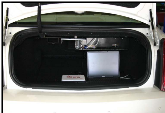
Figure 88 Data acquisition system, installed in the vehicle trunk underneath the rear shelf.
