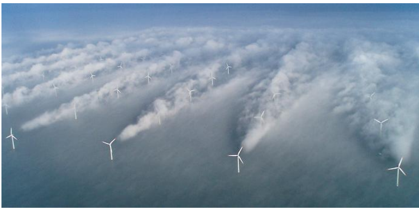
Horns Rev wind farm off the coast of Denmark. The wakes of the first row of turbines propagate and affect the downstream turbines. Picture used by permission of Uni-Fly A/S.
