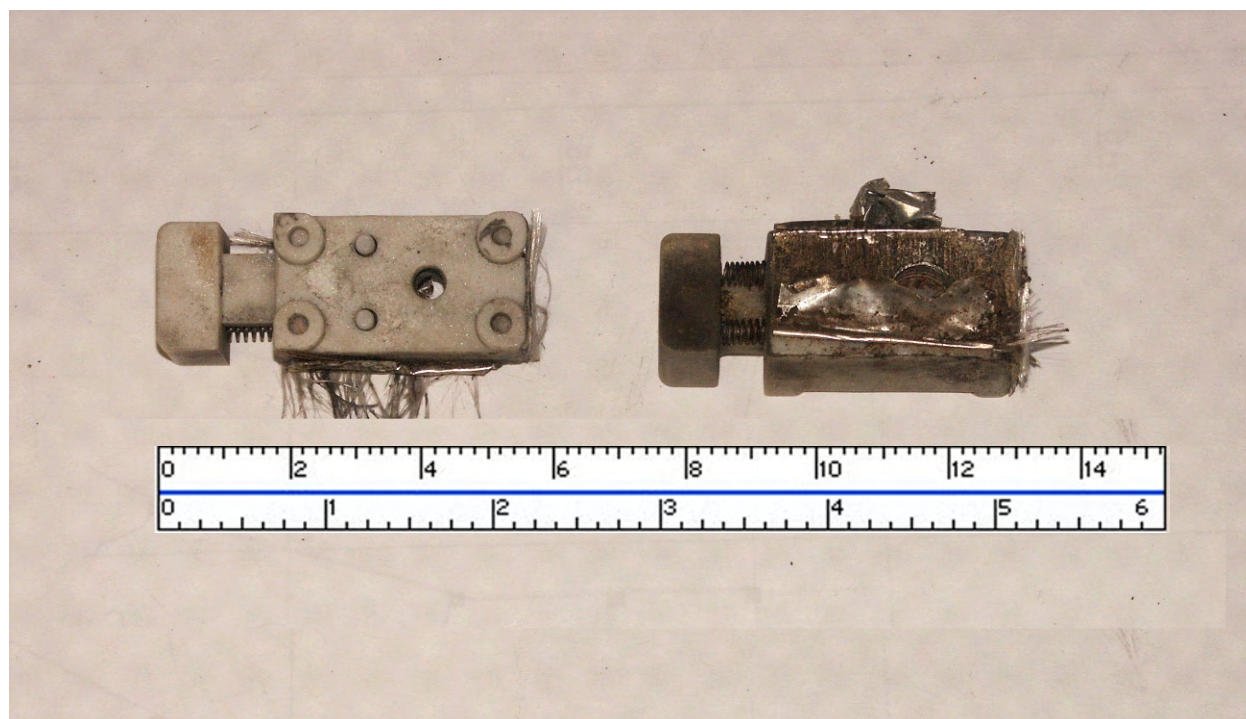
FIGURE 10. TWO S&I DEVICES USED IN MJU-7 A/B, AND OTHER FLARE TYPES
