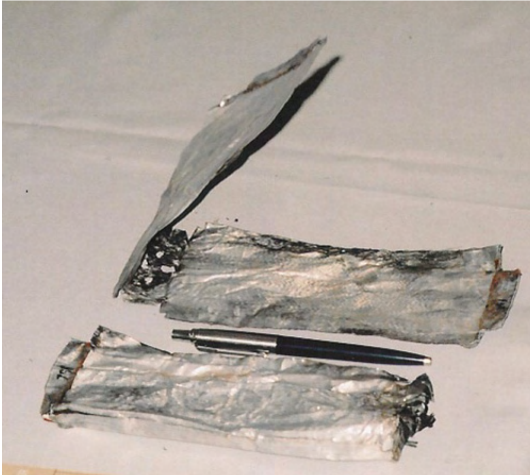
FIGURE 8. MJU-7 RESIDUAL FLARE WRAPPING MATERIALS
