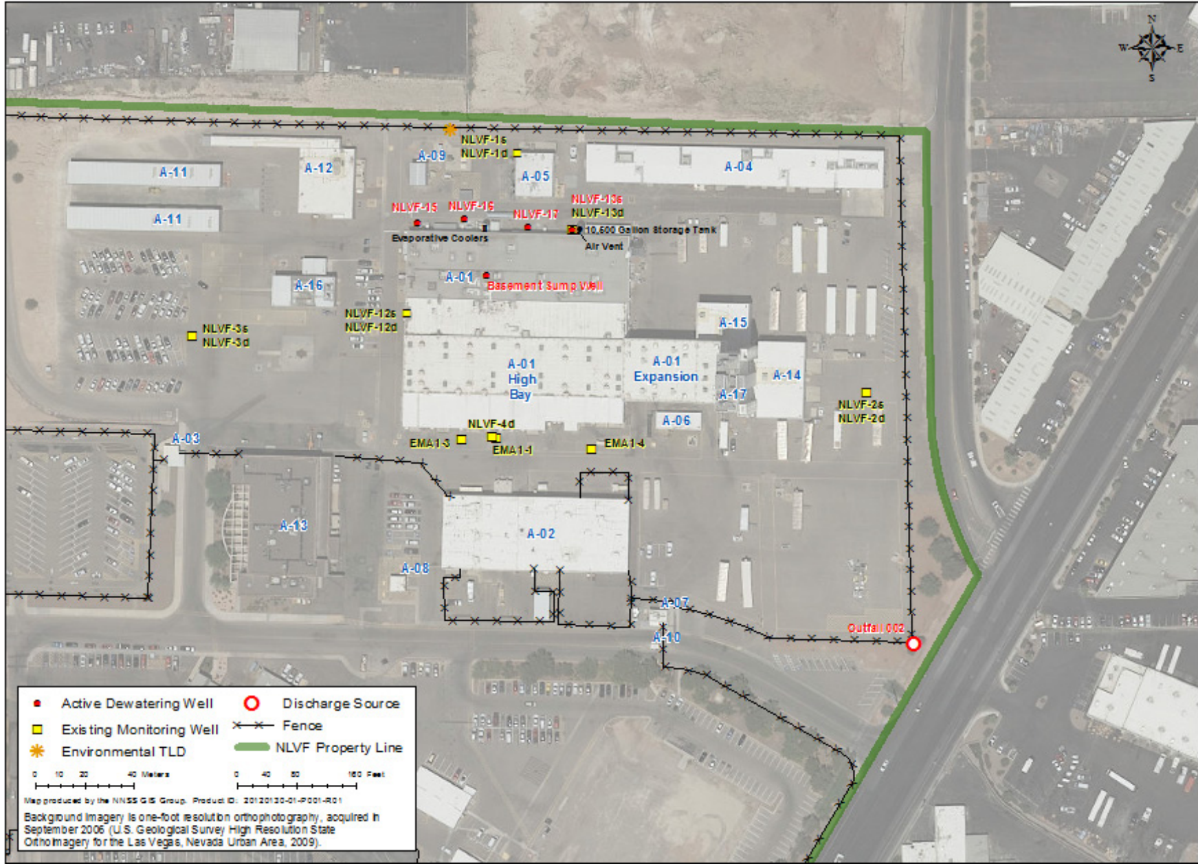
re A-2. Location of dewatering and monitoring wells around Building A-1
