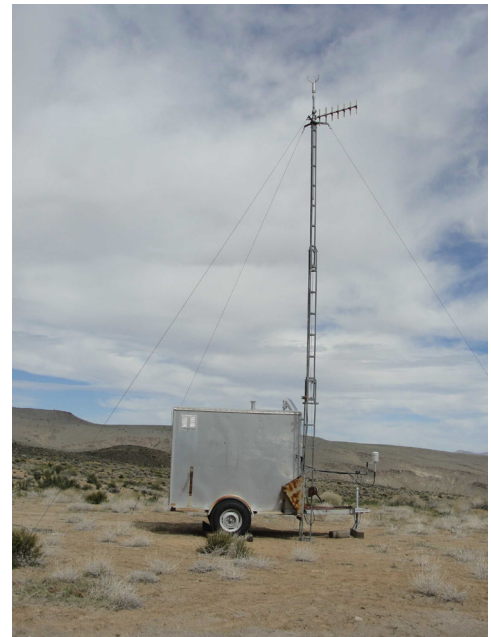
Figure A-12. Example of a typical MEDA station with a 10-meter tower
