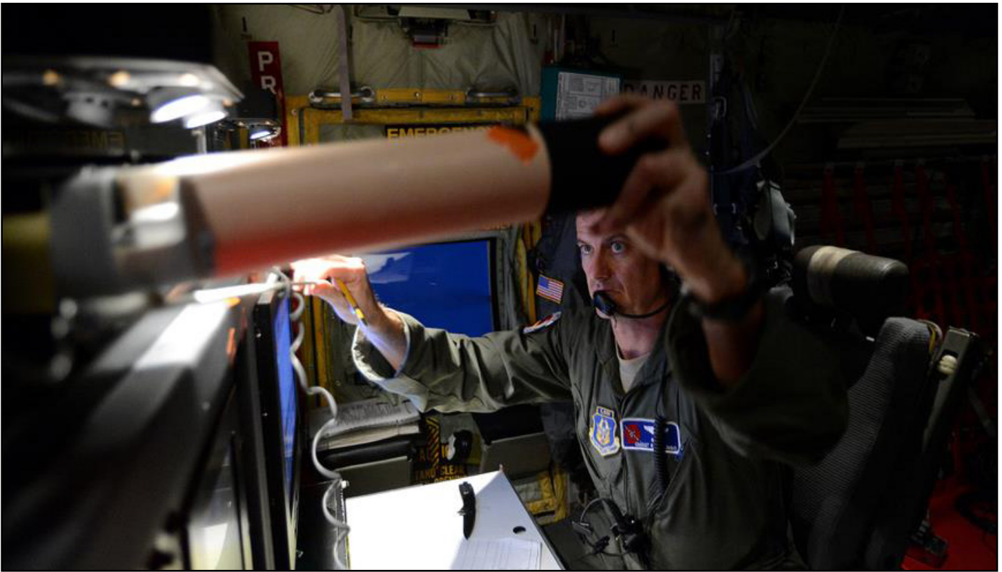
Chief Master Sgt. Rick Cumbo, a 53rd Weather Reconnaissance Squadron WC-130J Hercules loadmaster, prepares a drop sonde used to measure and transfer weather data back to the aircraft while flying into Hurricane Sandy Oct. 29 somewhere over the Eastern coastline. The drop sonde is ejected into the storm from the WC-130J using a specialized launcher, which then transmits real-time weather information back to the aircraft. (U.S. Air Force photo/Staff Sgt. Jason Robertson)
