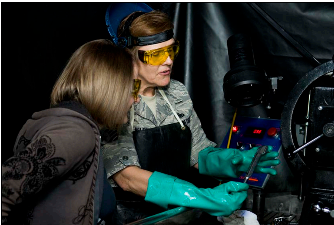
Master Sgt. Valerie Nelson, 434th Maintenance Squadron nondestructive inspection noncommissioned officer in charge, explains how to use magnetic particle inspection to find cracks in a main wheel rotor drive key to Cassie Dull, honorary Marine Corps Reserve commander, during a tour of Grissom maintenance Sept. 21. Dull was joined by Leilan McNally, honorary 434th Maintenance Group commander, and Jessica Green, honorary 434th Operations Group commander. (U.S. Air Force photos/Tech. Sgt. Mark Orders-Woempner)
