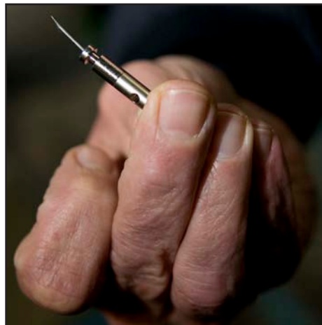
An electric probe of an electronic control device after firing it into a practice dummy.
