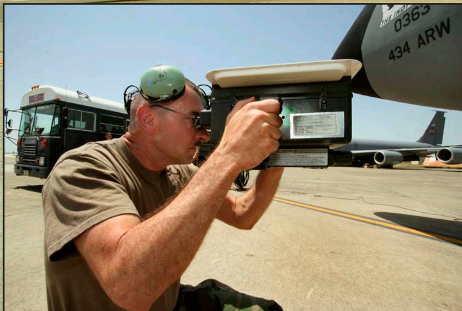
Tech. Sgt. Mark Wilson, 434th Aircraft Maintenance Squadron avionics guidance and control specialist, performs a check to ensure the friend or foe features on the KC-135R Stratotanker are operating correctly. This inspection is mandatory before the aircraft can depart.
